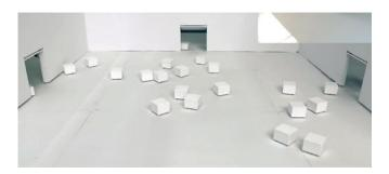
(**Dis)Appearables**, a project by MIT Tangible Media Group that explored the concept of cubical tangibles that are completely mobile and can move on their own. They are controlled by a central unit and can visualize or express content by appearing and disappearing from a stage.
