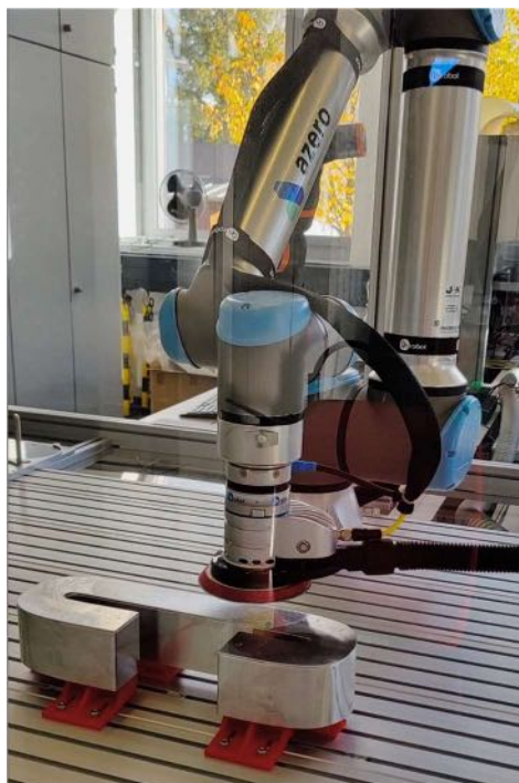
Figure 1: robot cell with object to be polished
