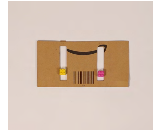
4. Sliders : One slider for each player to move the paddle up and down. The position of the slider element represents the absolute position of the striker paddle.
