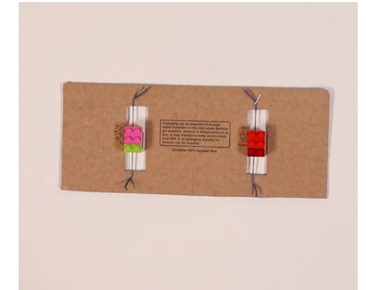
5. Velocity shifters : One shifter for each player. A sliding element is attached to a rubber band for haptic force feedback. This interface controls the velocity of the striker paddle in each direction.
