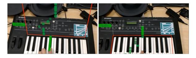
For mode A, visual feedback is given to the user by highlighting the played keys in a colour indicating how precise he played the note (green: good, yellow: medium, red: bad). For mode B, this feedback is displayed in another position, which is at the upper edge of the keys, as it would overlap with the moving panels indicating notes.
