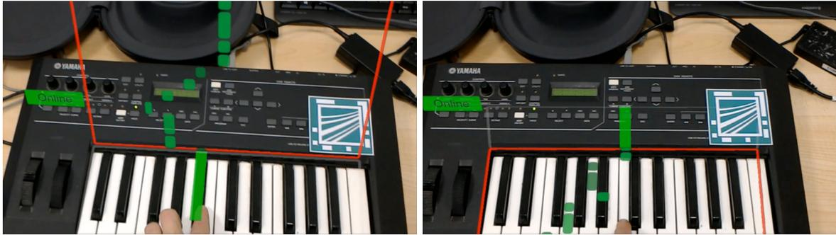
For mode A, visual feedback is given to the user by highlighting the played keys in a colour indicating how precise he played the note (green: good, yellow: medium, red: bad). For mode B, this feedback is displayed in another position, which is at the upper edge of the keys, as it would overlap with the moving panels indicating notes.
