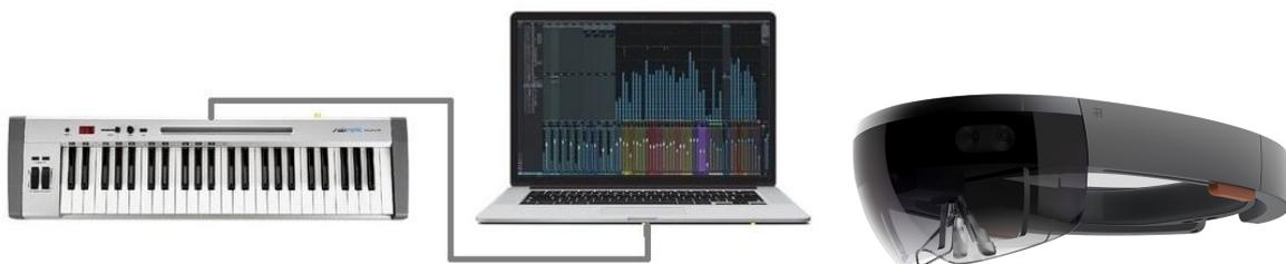
For the visual output of musical notation and key feedback, the Optical See-Through Displays (OSTs) of Microsoft HoloLens are used.
