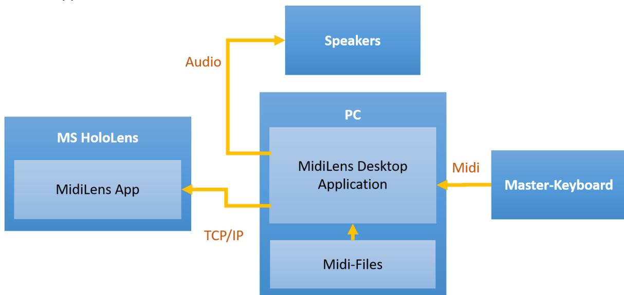
The MidiLens Desktop Application which was written in C# and mostly serves as an interface between the technical components. Its main functions are:
